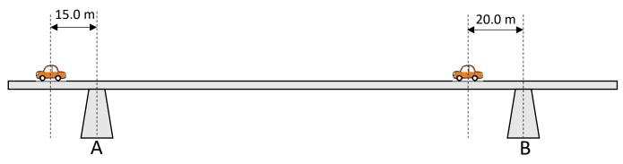
(a) Calculate the magnitude of the force that pillar A exerts on the bridge when two 8.00 kN cars are located at the positions shown.
